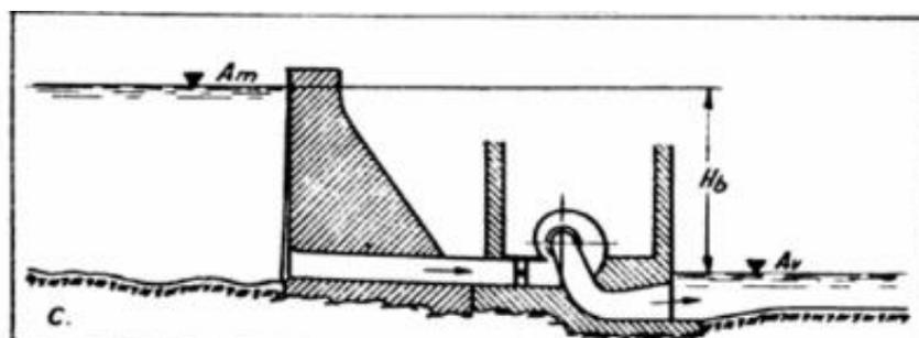
Figure 2.2 - The gross fall of the arrangement of the hydroelectric plant with a Pelton turbine.
