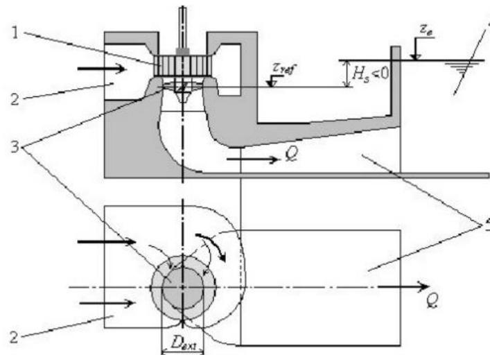
Figure 1.21 – Schematic of the Kaplan turbine: (1) stator; (2) concrete semi-spiral chamber; (3) rotor with adjustable blades; (4) discharge basin; (5) crank vacuum cleaner
