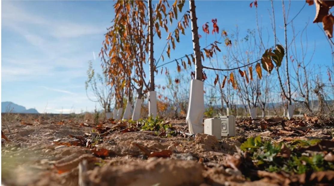
*Figura 13 Installation of humidity sensors, at two different levels Comunidad de Regantes de Pliego*
