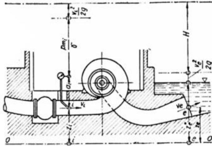
Figure 2.1 - Input and output parameters for the Francis turbine.
