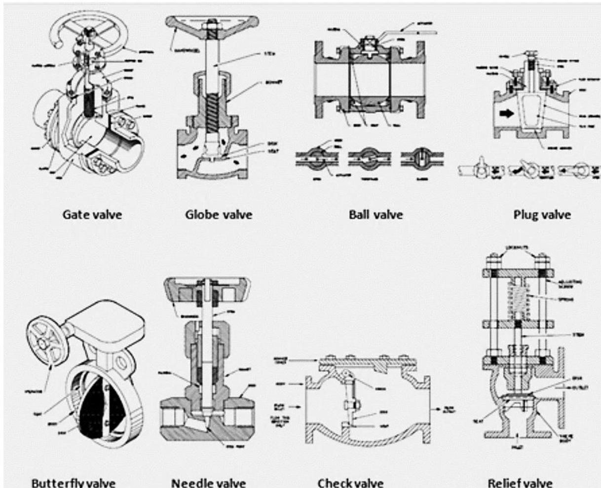
*Figure 1.24 - The main types of valves*
