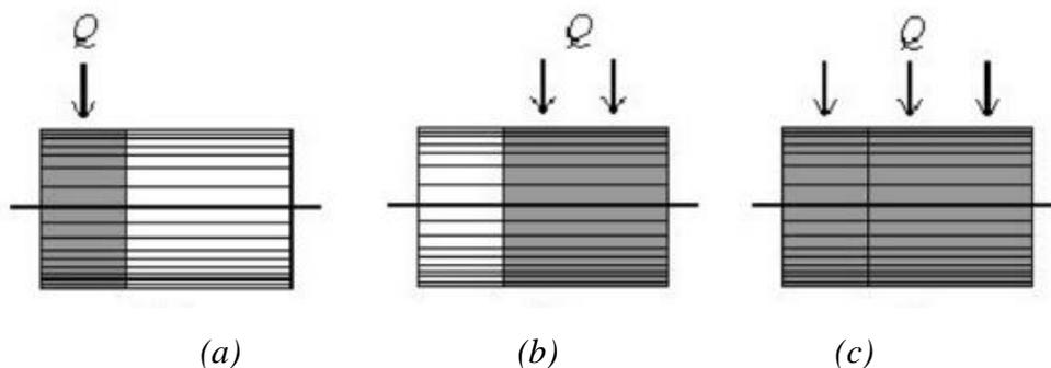
Figure 1.12 - Ossberger-Michell turbine rotor compartmentation, for: (a) low flow rates; (b) average flows; (c) high flows
