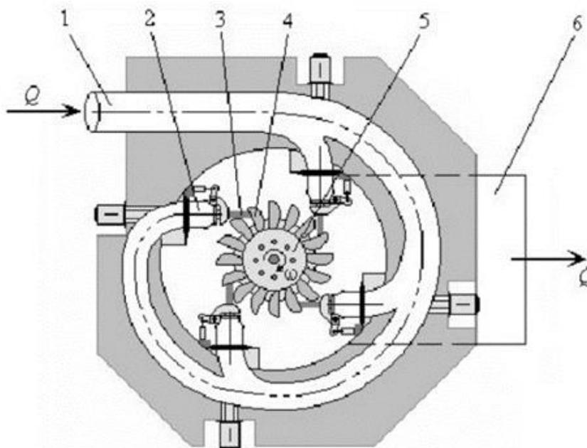
*Figure 1.9 - Pelton turbine diagram with 4 injectors: (1) supply pipe; (2) injector; (3) water jet; (4) rotor bucket; (5) rotor; (6) discharge basin*
