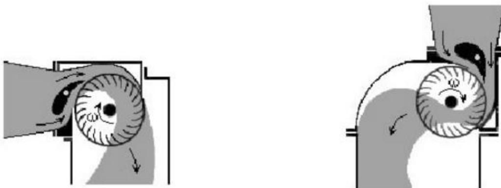
*Figure 1.10 - Bánki turbine (Ossberger-Michell): (a) water intake in the horizontal direction; (b) vertical water inlet*
