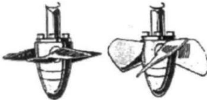
*Figure 1.19 - Extreme positions of the rotor blades of a Kaplan turbine*
