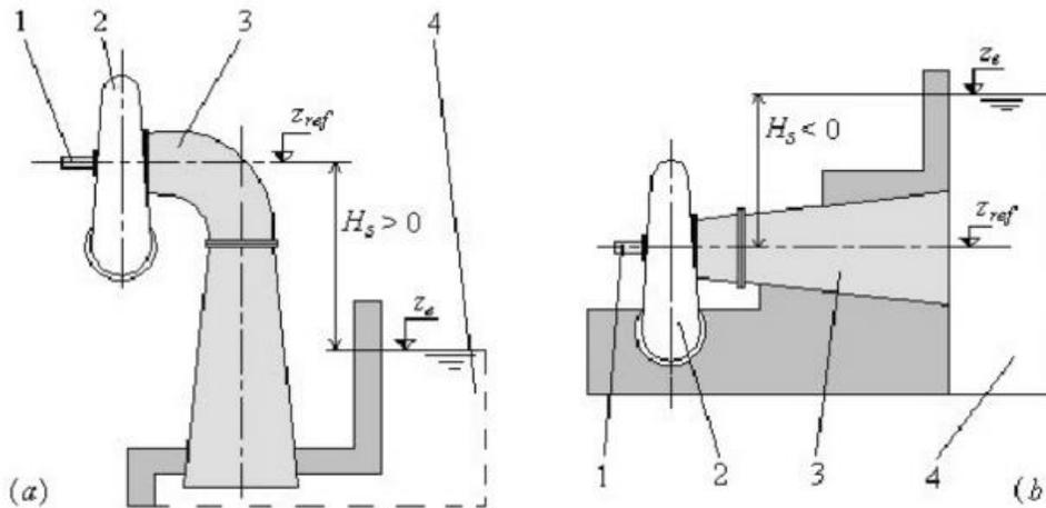
Figure 1.18 – Francis turbine with horizontal shaft (a) with cranked suction; (b) with rectilinear vacuum cleaner: (1) shaft; (2) metallic spiral chamber; (3) vacuum cleaner; (4) discharge basin
