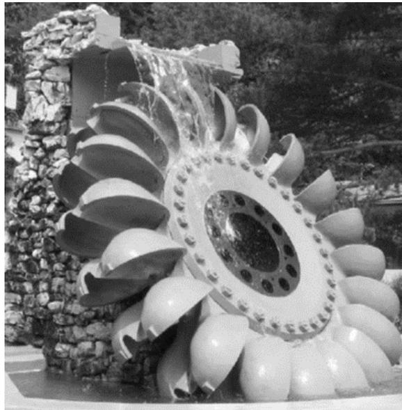
*Figure 1.6 - Pelton turbine rotor [Lotru Ciunget Hydroelectric Power Plant, July 2003]*
