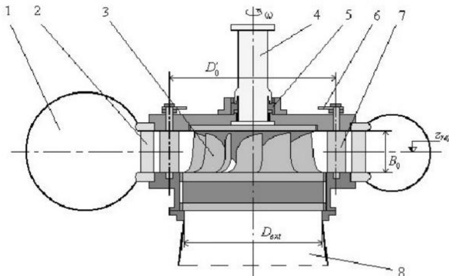
Figure 1.15 – Normal Francis turbine: (1) metallic spiral chamber; (2) stator; (3) rotor; (4) vertical shaft; (5) radial bearing; (6) operating mechanism of the steering device; (7) radial steering device; (8) crank vacuum cleaner
