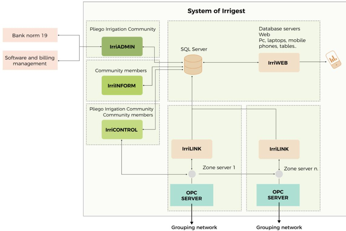
*Figura 16 Irrigest system applied in the Irrigation Community of Pliego*
