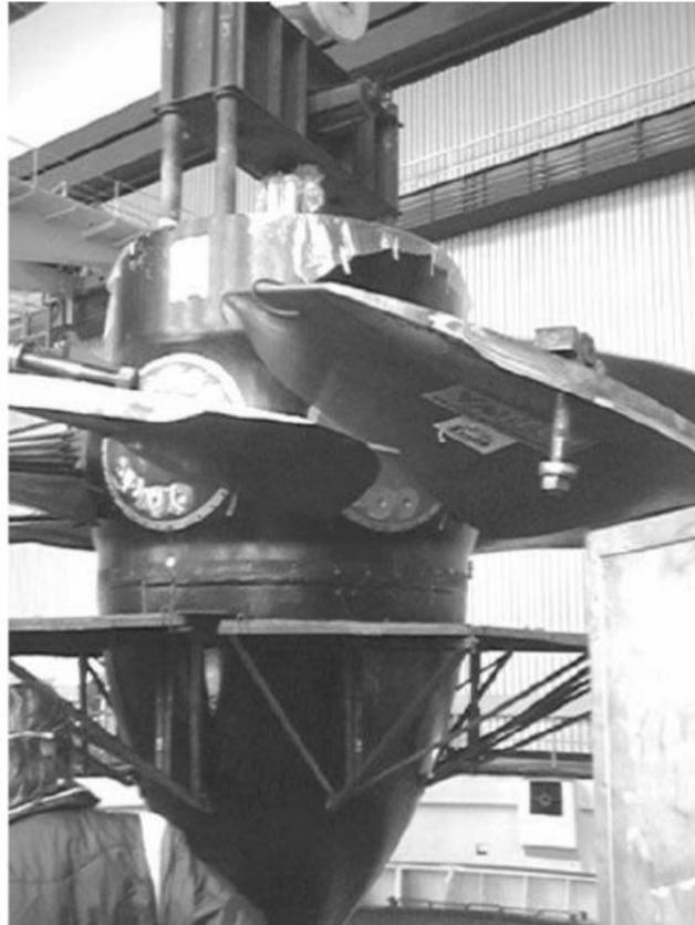
*Figure 1.20 – The rotor of the Kaplan turbine [Hydroelectric power station "Iron Gates I", May 2003]*
