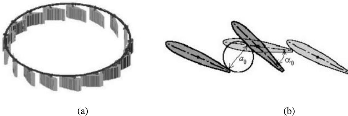
Figure 1.17 – Direction device: (a) direction blades caught by the adjustment ring, in the open position; (b) defining the opening angle of the steering apparatus blade in the open position, respectively the presentation of the blades in the closed position
