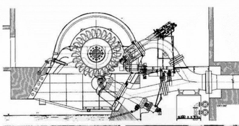
*Figure 1.8 - Hydroelectric installation with a Pelton turbine*
