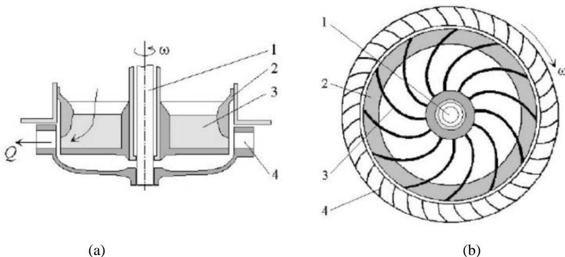
*Figure 1.13 - Fourneyron turbine in (a) cross section and (b) parallel plane view: (1) shaft; (2) cylindrical valve; (3) steering blade; (4) rotor blade*
