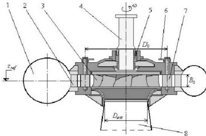
Figure 1.14 – Slow Francis turbine: (1) metallic spiral chamber; (2) stator; (3) rotor; (4) vertical shaft; (5) radial bearing; (6) operating mechanism of the steering device; (7) radial steering device; (8) crank vacuum cleaner
