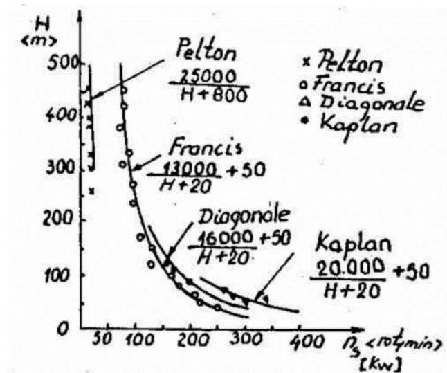
Figure 2.3 - The relationship between the critical specific speed at a global suction height
