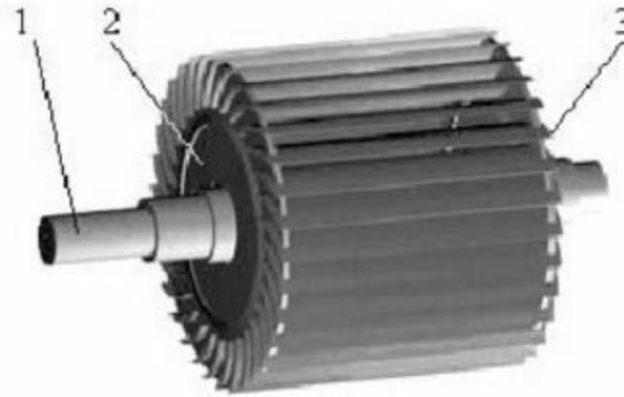
Figure 1.11 - Bánki turbine rotor: (1) shaft; (2) circular blade support disc; (3) horizontal blade, simply curved
