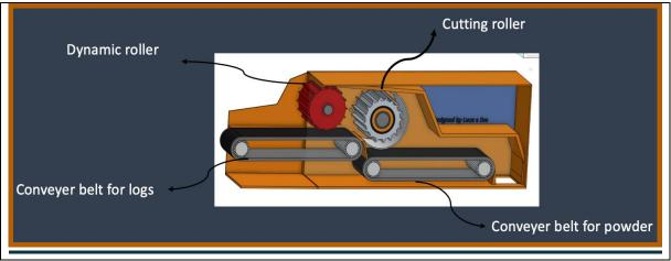
Second model of wood chopping machine [fig2.2.9]
