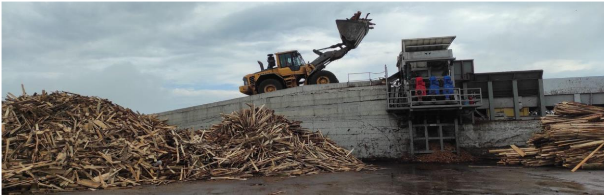
Figure 8. Heavy machinery loading wood into the chipper.
