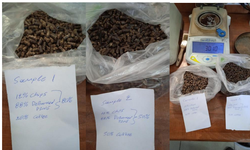
Figure 13. Sample 1 made with 20% SGC and with 80% wood mix and sample 2 made with 50% SGC and 50% wood mix.
