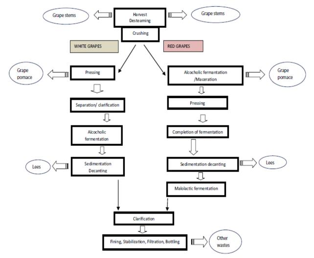
Figure 3.3. Grape by-products generation during wine production process (Kalli et al., 2018)
