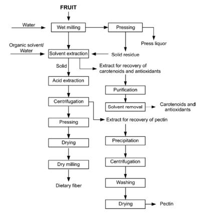
Figure 5.5. Flow diagram for the utilization of fruit pomace (Khgk and Rauj, 2017)
