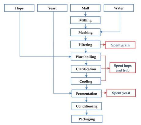
Figure 4.2 Schematic representation of the brewing process and points where the main by-products are generated (Karlović et al., 2020)
