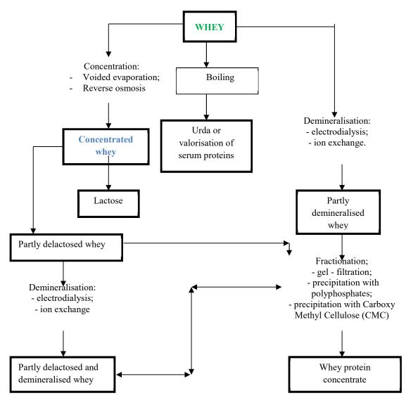
Figure 2.5 Processes for fractionating the dry substance from whey (Azzouz, 2002)
